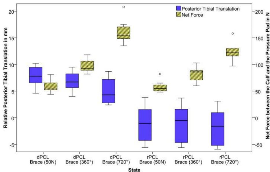
**Fig. 4.** Comparison of posterior tibial translation (blue boxes) relative to the native knee and the net force between the calf and the posterior pressure pad (hatched yellow boxes) using the brace with an initial anteriorly directed force applied (50 N) and increased anteriorly directed forces by turning the wire traction wheel of the pressure pad by one and two full turns (360°, 720°). dPCL, dissected posterior cruciate ligament; rPCL, reconstructed posterior cruciate ligament.
